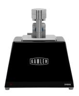
Make the tablets using the Gamlen D1000 or D500. Maximum compaction load for the D1000 is 1000 kg and 500 kg for the D500. The D500 is recommended for minitabs.
