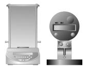
Tablet thickness and mass are measured using a micrometer and balance.
